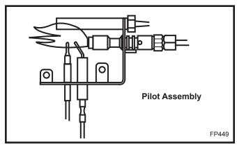
Fig. 19 Proper pilot flame height.
